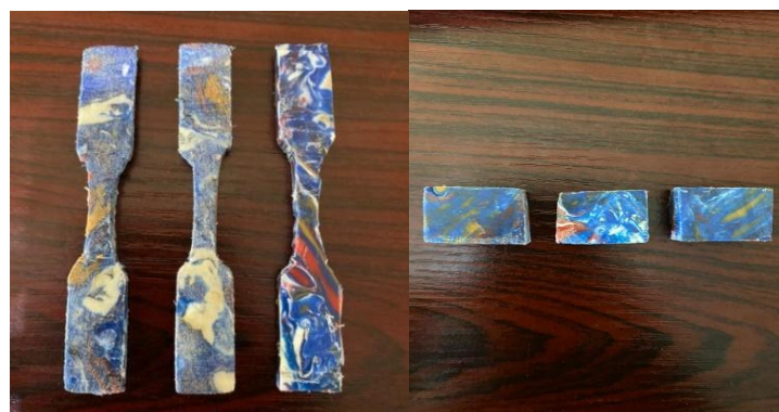
Fig. 11. Prepared plastic recycle for testing.
