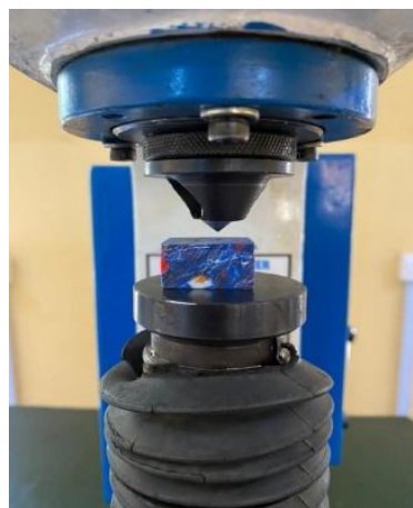
Fig. 14. Specimen readied for Rockwell hardness test.
