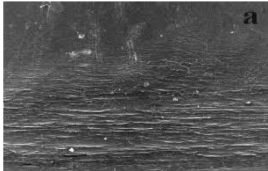
Fig. 22. SEM image for virgin HDPE plastic.
